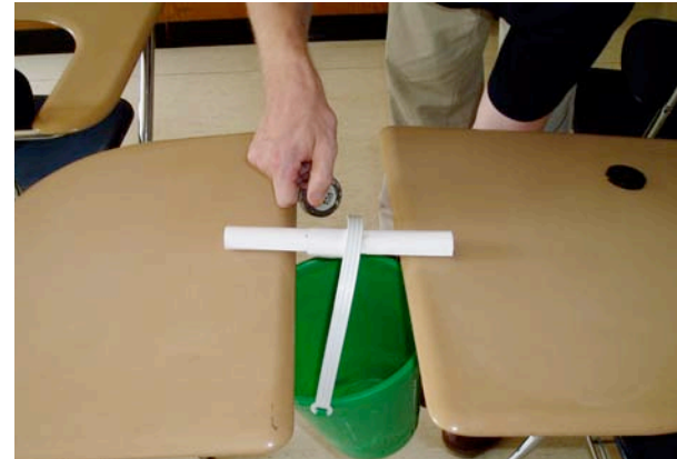
Figure 1: Loading the bone construct for strength testing.
