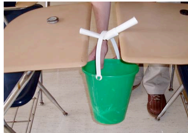
Figure 2: Quantifying bone construct strength. Structural failure upon critical load.
